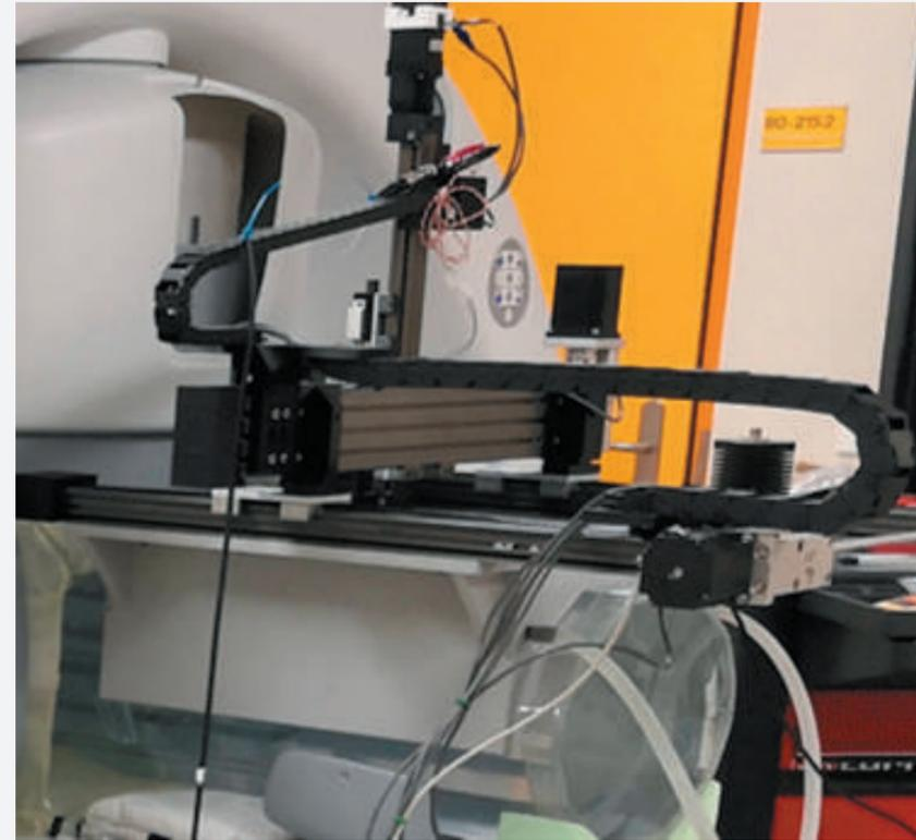
3D E-field measurement phantom is used for Hyperthermia device QA tests of:
